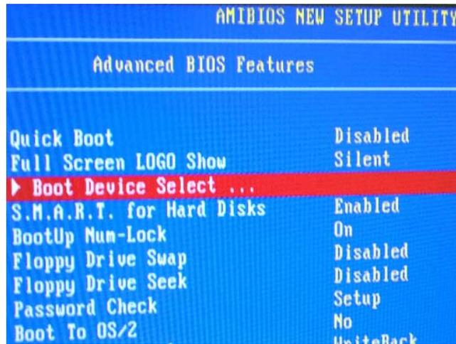
7. Select **USB RMD-FDD Generic STORAGE DEVICE** for the 1st Boot Device, then press **ESC**.
